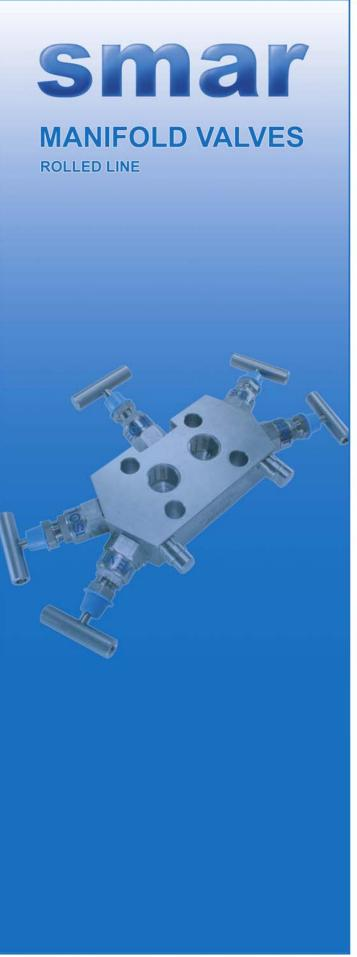
Smar rolled valves line is made up of Block Valve, 2, 3 and 5-way Manifold Valves. They are tipically produced in rolled 316 SST but optionally also in Hastelloy\*, Treated Carbon Steel\*, Monel\* and Super Duplex\*. Their design adopts the needle type valve concept for high pressures with a non-rotating shutter, which provides high air-tightness to the process.
